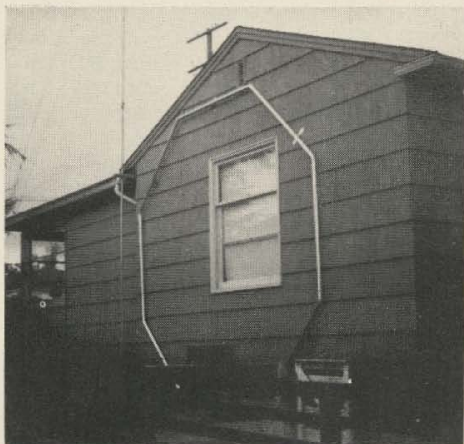
The Ferris Wheel antenna mounted to the side of WA7CUS's house.
